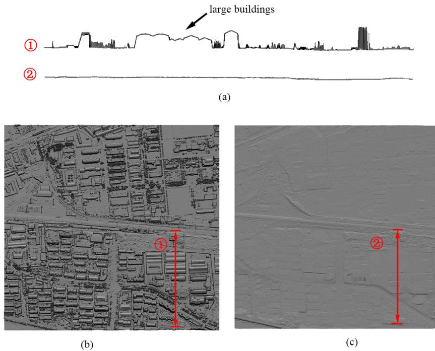
**Figure 9.** Removal of large buildings in urban area: (a) Cross sections from (b) and (c); (b) Dataset 1; (c) Produced DTM. In this dataset, it contains a number of connected large low buildings (see the cross section), when the cloth is relatively hard, it will not drop into this large hole, then these buildings can be removed.
