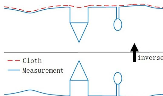
**Figure 1.** Overview of the cloth simulation algorithm.
