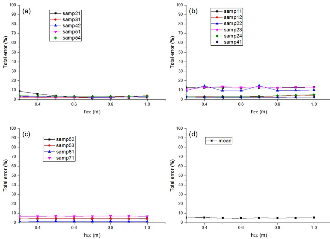
Figure 15. The influences of  $h_{cc}$  on total errors: Group I (a); Group II (b); Group III (c); Mean (d).
