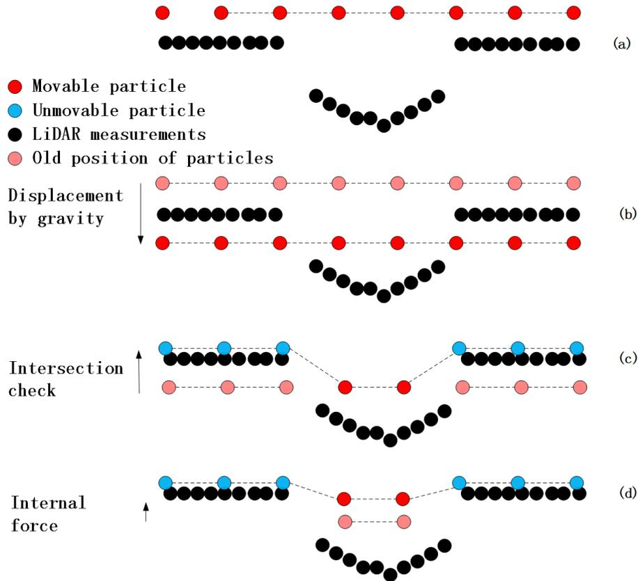
**Figure 3.** Main Steps in CSF: (a) Initial state. A cloth is placed above the inverted LiDAR measurements; (b) The displacement of each particle is calculated under the influence of gravity. Thus, some particles may appear under the ground measurements; (c) Intersection check. For those who are under the ground, they are moved on the ground and set as unmovable; (d) Considering internal forces. The movable particles are moved according to forces produced by neighbour particles.
