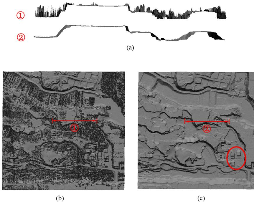
**Figure 12.** Preservation of steep slopes: (a) Cross sections from (b) and (c); (b) Dataset 4; (c) Produced DTM. In this dataset, the main objects are vegetation and contains large number of ground measurements, the cloth can be very soft to maximumly fit the terrain shape with less consideration of T.II error. Companied with post-processing, large steep slopes can be preserved well.
