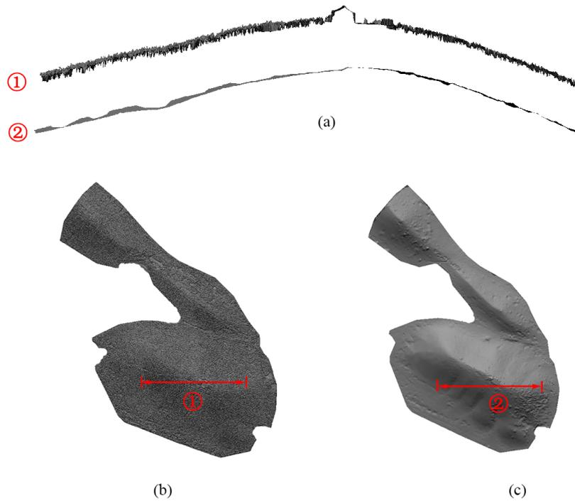
**Figure 11.** Sparse ground measurements: (a) Cross sections from (b) and (c); (b) Dataset 3; (c) Produced DTM. In some hilly topography areas, some parts of the cloth may not sticks to the ground well, this will cause classification errors (BE may be treated as OBJ).
