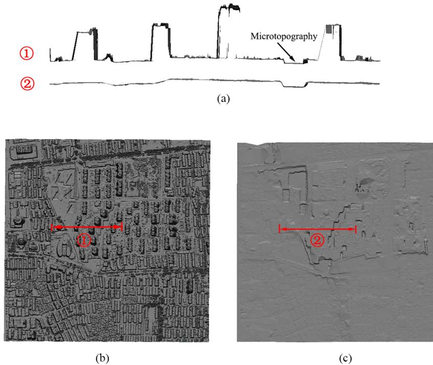
**Figure 10.** Preservation of microtopography: (a) Cross sections from (b) and (c); (b) Dataset 2; (c) Produced DTM. When post-processing is enabled, the cloth can stick to the surface more closely, some small steep slopes can be preserved.
