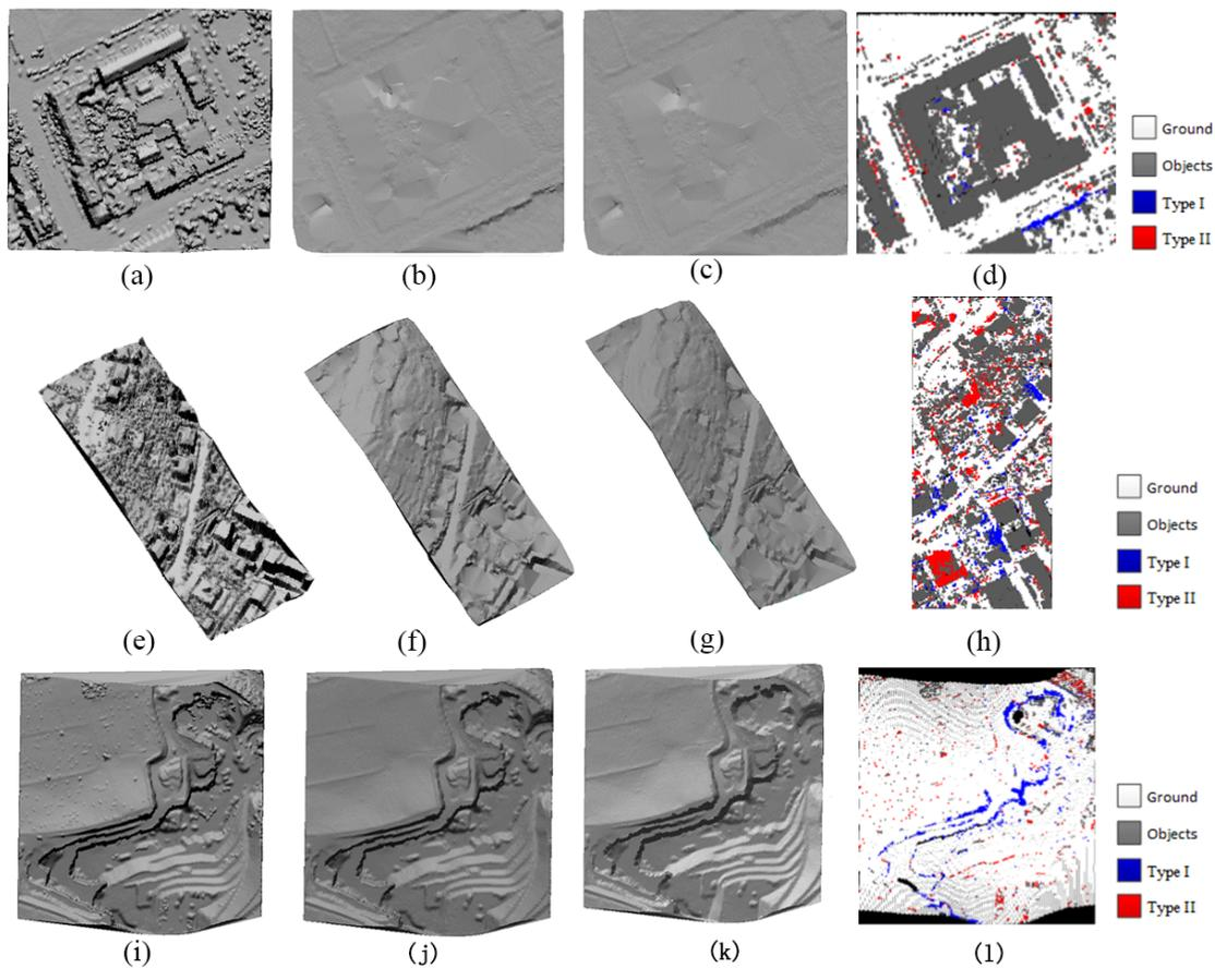
**Figure 8.** Results of each group (choose samp31, samp11, and samp53 as representatives): **(the first column)** are original datasets; **(the second column)** are the DTMs that are generated from the reference data of samp31, samp11, and samp53; **(the third column)** are the DTMs that are produced from the CSF algorithm; **(the last column)** are the spatial distributions of the type I and type II errors.
